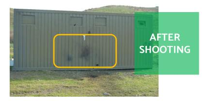
Container Type : Weapon/Ammo Type: Range : Housing, made of prefabric material 40 mm Projectile 50 m
